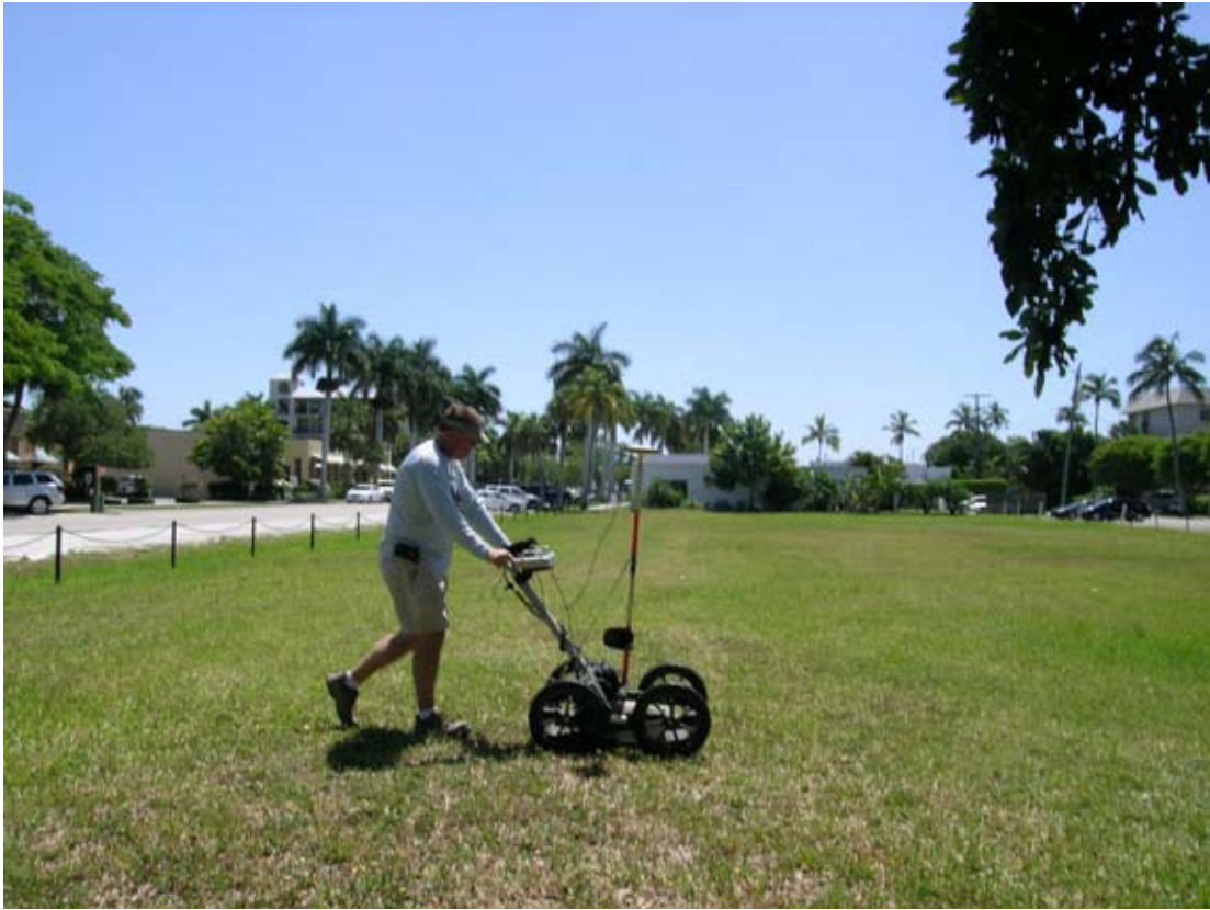
Figure 7. GPR scanning conducted at Location 1, east end of canal.
