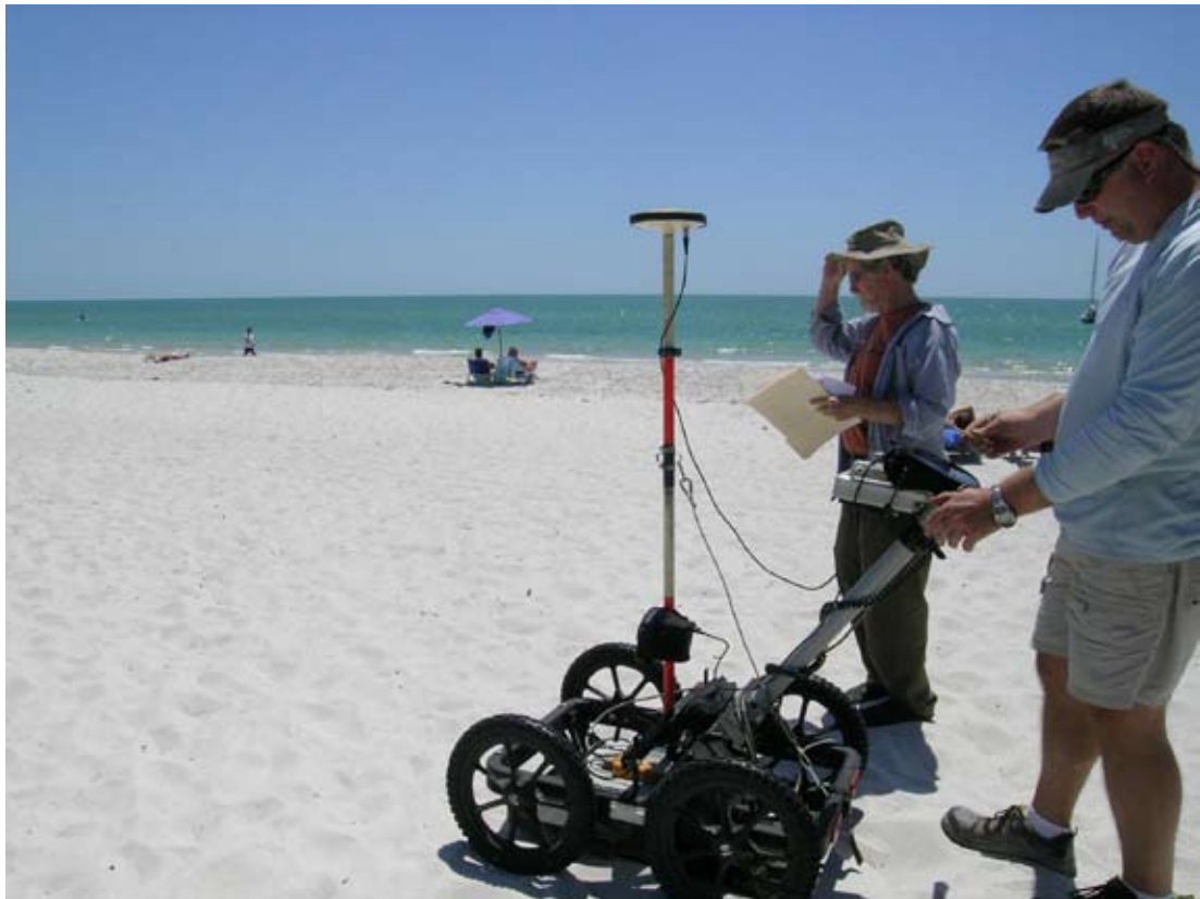
Figure 8. GPR scanning conducted at Location 7, west end of canal.
